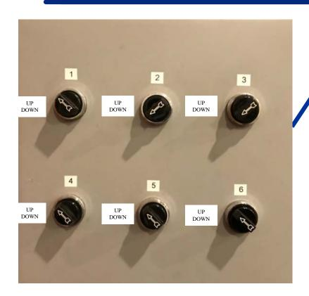
Activating the switch raises and lowers the barrels via pneumatics
