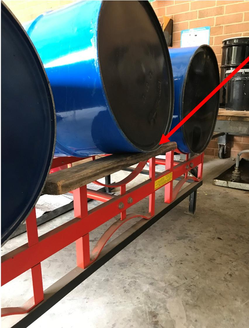
In the past when a drum was almost empty, EE would lift the barrel and place a board under the tote to raise the drum to empty the content
