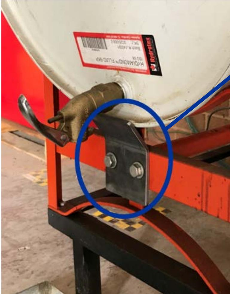
EE came up with the idea to add a safety ledge to the front side of the barrel rack to keep the barrels from sliding off when lifted
